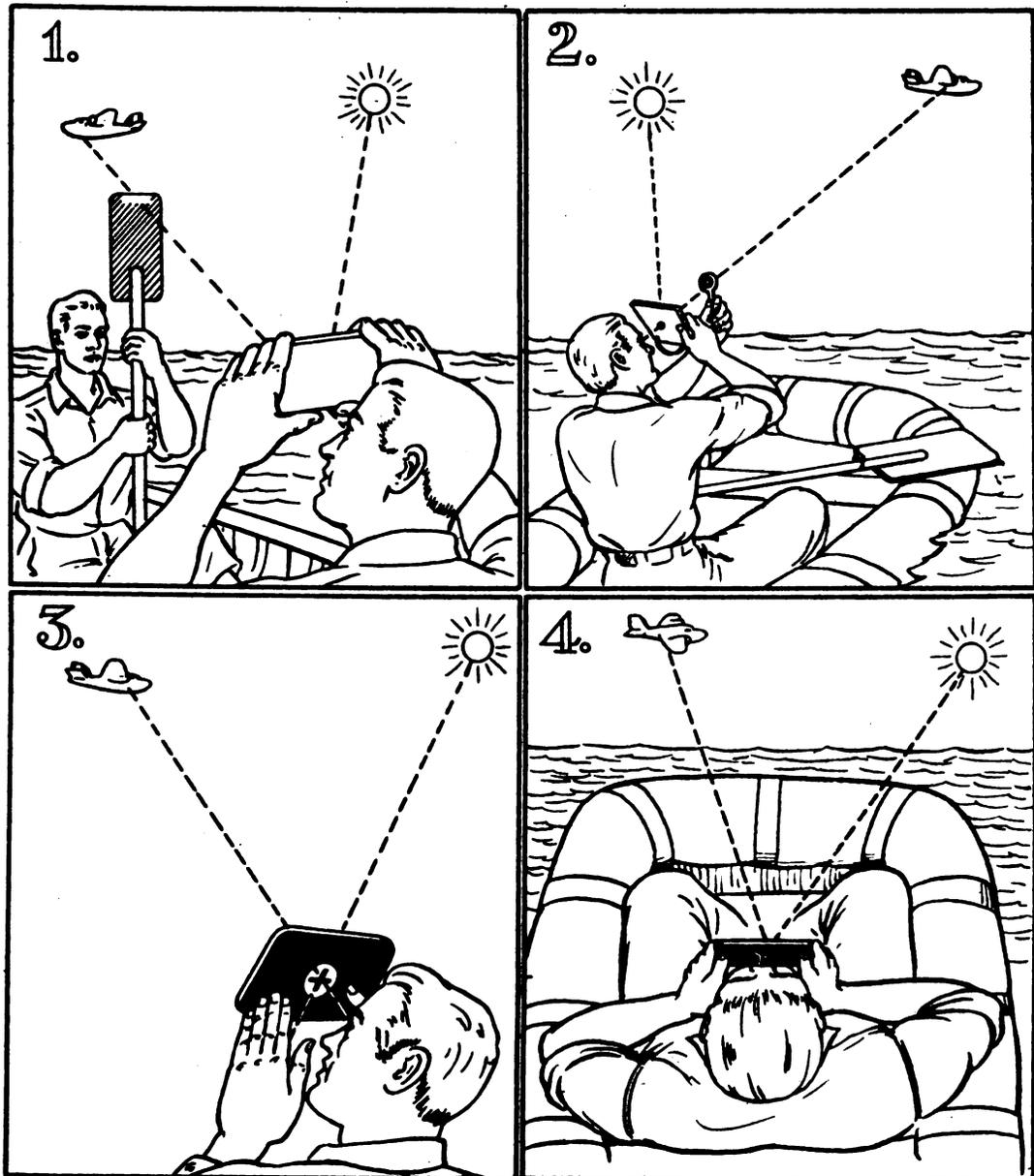
Figure 2. Diagram illustrating four methods of aiming mirror flashes of sunlight: (1) Sighting surface, (2) Foresight (British mirror), (3) Rearsight (G. E. mirror), and (4) Reflex button.
