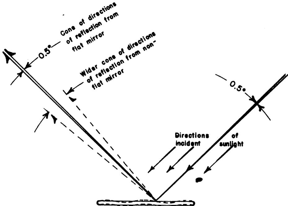
Figure 1. Diagram showing the directions of reflection of sunlight from flat and non-flat mirrors
